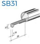
Code 1.705 For planes and holes. Hole Ø minimum 4 mm max depth 20 mm.
