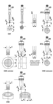
special probes OSIMESS OSF
