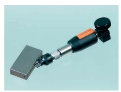
OSF special probe for keyway
