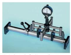
ESU Setting Device for OD cross sleeves/ cross sleeve with runners
