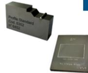
The standard equipment includes the one area roughness calibration specimen (code: 6.103). The profile kit, instead, includes the probe and the specimen dedicated to measuring and calibrating the profiles (codes: 2.503 + 6.302).
