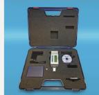
Roughness tester RT10 or RT10G combined with probe SB 10 Battery charger unit 110-220V Positioning supports
