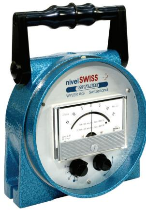
Battery powered electronic inclinometer with analog display on a built-in galvanometer. The remarkable stability of the zero-point makes this instrument particularly suitable for long-term measuring tasks and for adjustment or alignment works on large guideways. The nivelsWISS is mounted in a rugged body of carefully treated cast iron.
