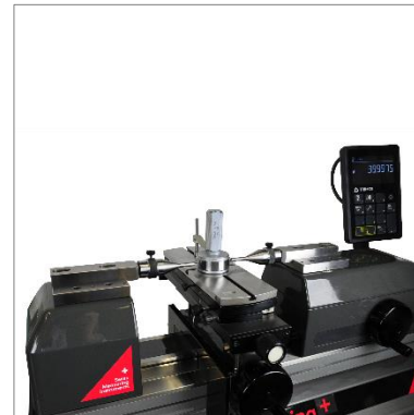
Checking of plug gauges (larger than dia. 100mm) (TEL6, TA-SU-313, TULM6/L0.5, TA-SU-304)
