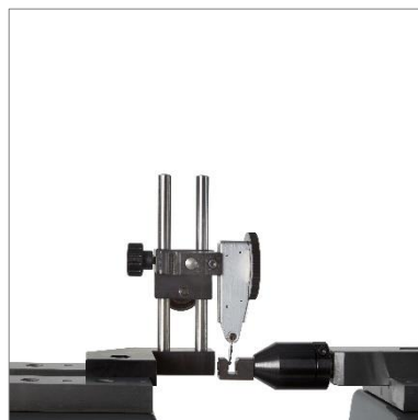
Checking of test indicators (TULM 15.1)
