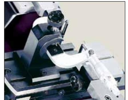
Checking of external micrometers (HPA-1/TULM14)
