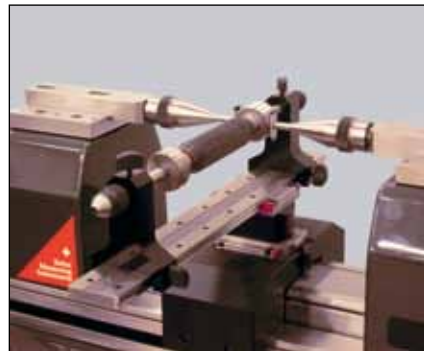
Checking of thread plug gauges (HPA-1/TEL6/3P/0.17-3.2/S6.5/LABC-15)
