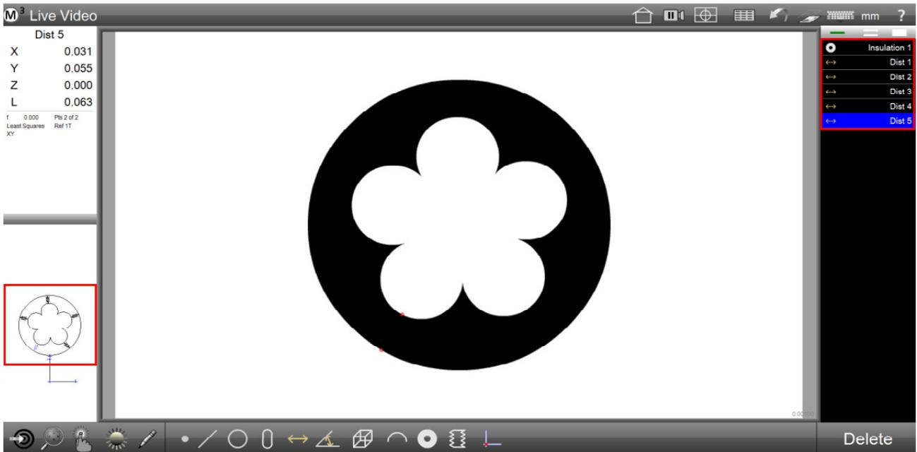
Thanks to the **Smart\_Wire\_Measurement** insulation tool it is possible to determine the number of strands in a wire automatically, as well as manually select the appropriate figure.
