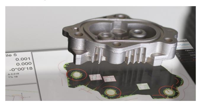
Smart\_Profile\_Matching is an **automatic Profile Check advanced feature**, which can control any item compared to a DXF master. This feature replaces the use of a traditional profile projector that requires the overlay of a glossy sheet on the component's projection.
