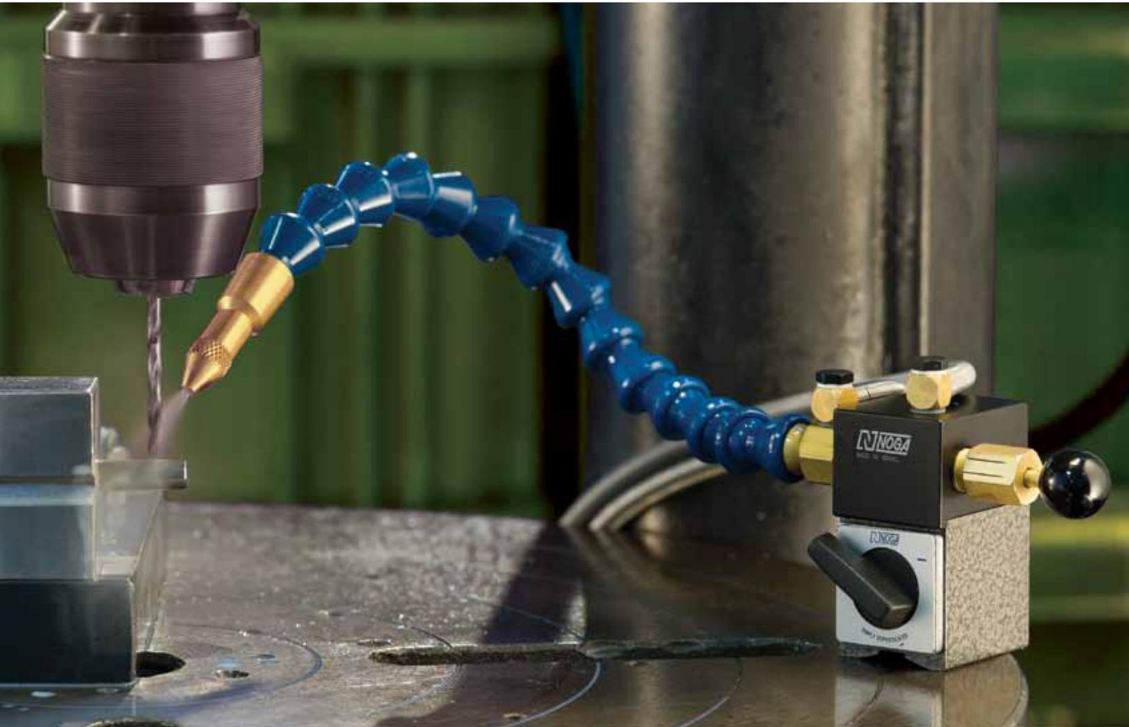
**NOGA MINICOOL** uses the VENTURI principle to spray an air and liquid mixture. It consists of the following basic parts:
