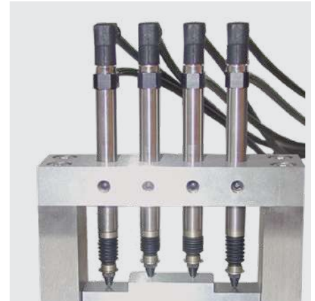
Combined probes for the measurement of several heights
