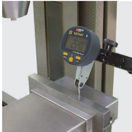
Checking the alignment on milling machine.
