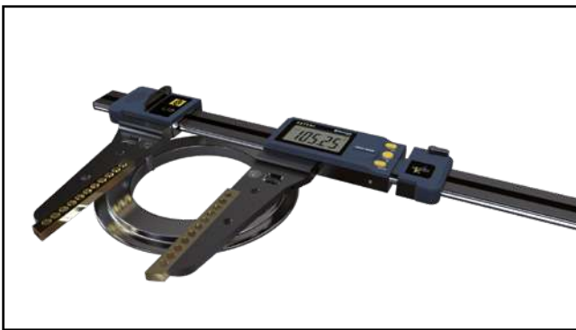
Internal measure with UL4
