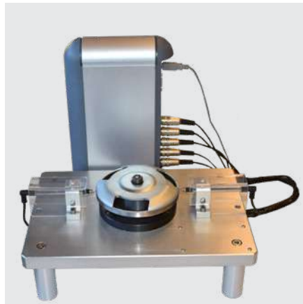
Capacitive probes connected to a D200S.
