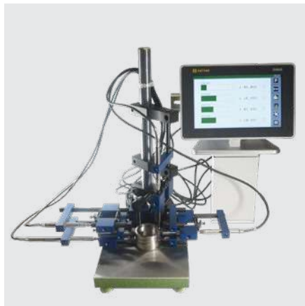
Inductive probes connection on a jig
