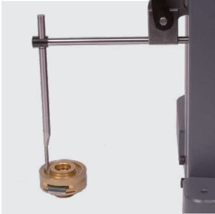
Depth measurement with accessories 930-2108 and 930-2105
