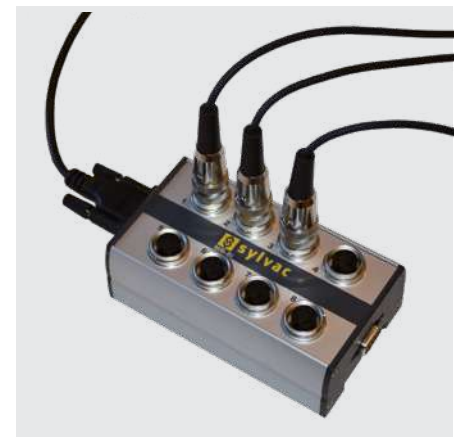
Probes connected to an MB-8i
