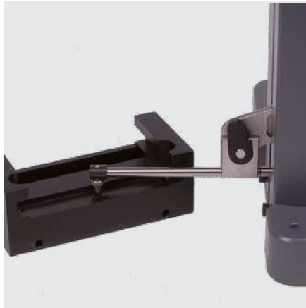
Depth measurement with accessories 930-2108 and 905-2204
