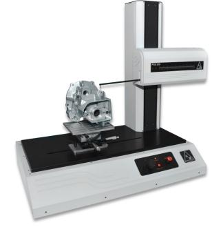
The PGS200 profilometer is a new concept instrument able, with a few simple operations, to characterize the profile even of more complex details and thanks to the modern "all in one" philosophy, it is immediately operational to carry out the measurements.
