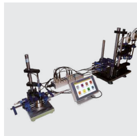
Probes and indicators connection through M-BUS inputs
