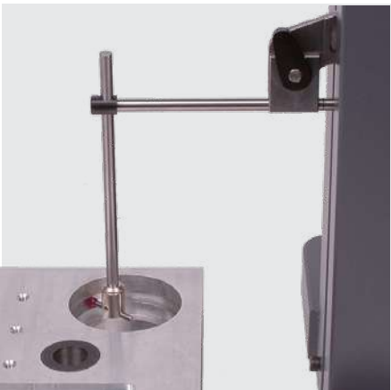
Internal groove measurement with accessories 930-2108, 930-2110 and 905-2207
